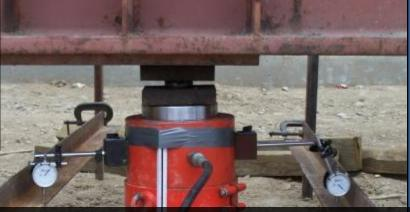
Load tests passed with good results. Measured 0.28 inches movement at 110 kips design compression and tension loads. Installation was completed on budget and on schedule.
