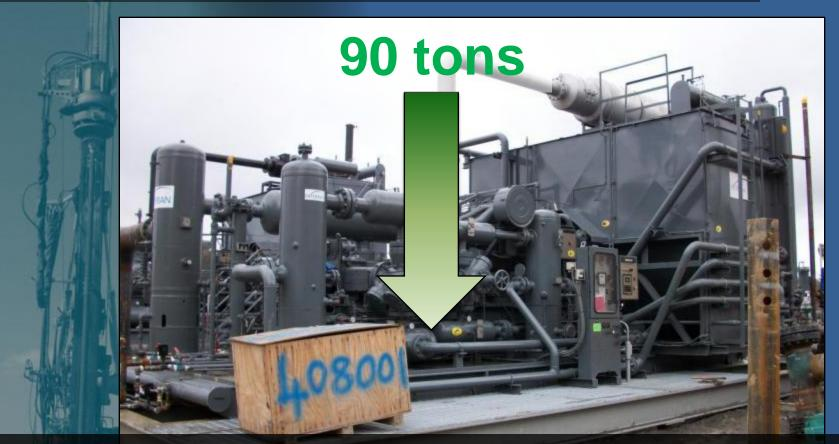
Designing the foundations for vibrating machines is not as simple as dividing the weight amongst the piles. The lifespan and maintenance cycle of compressors and other machines is greatly diminished with improper foundation design and excessive vibrations.
